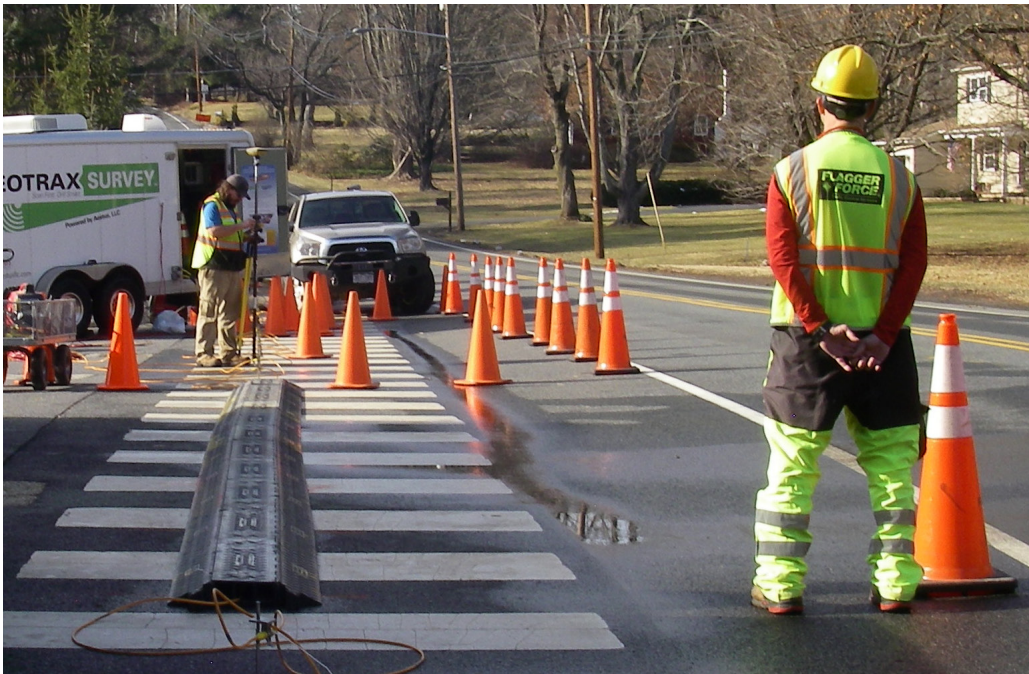
GeoTrax Survey™ transect with traffic ramps over electrodes and cables; allows traffic to flow unimpeded
