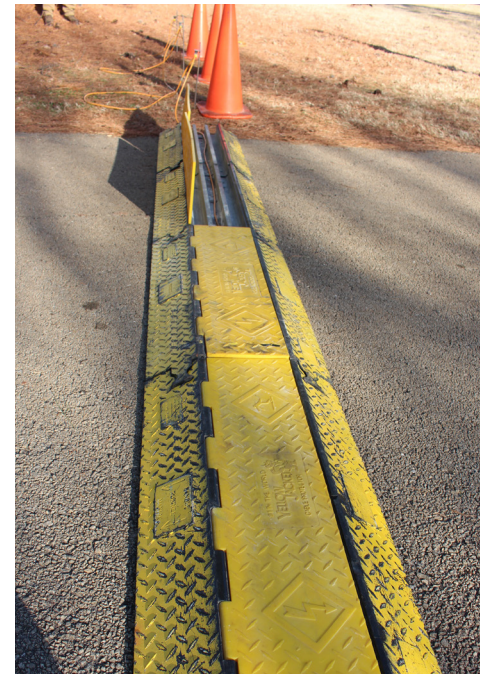
GeoTrax Survey™ transect with traffic ramps over electrodes and cables; allows traffic to flow unimpeded
