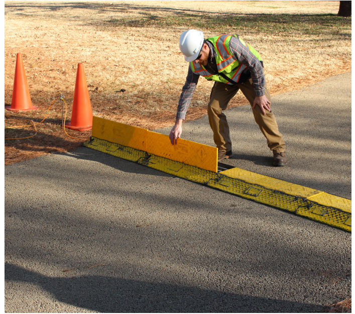
GeoTrax Survey™ transect with electrode stakes in pre-drilled 1/2-inch diameter holes through asphalt pavement.
