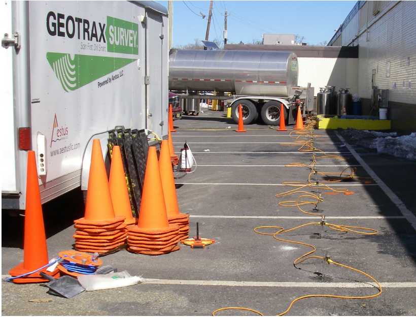
GeoTrax Survey™ transect with electrode stakes in pre-drilled 1/2-inch diameter holes through asphalt pavement.
