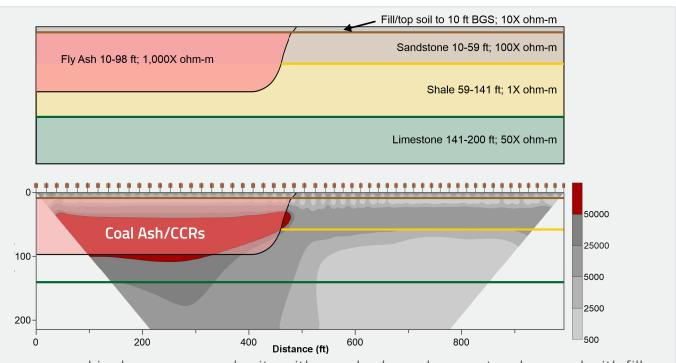
The upper graphic shows an example site with a coal ash emplacement and covered with fill material, resulting in no discernible ash lateral boundary on the ground surface. The lower graphic depicts what would be seen in the resulting GeoTrax Survey™ scan. Notice how the lateral extent and bottom of the fly ash deposit are clearly visible as a distinct, strong electrically resistive anomaly (dark red zone in image).
