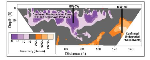
Aestus integrated historical and targeted confirmation drilling data onto our GeoTrax Survey™ 2D subsurface images as well as our 3D visualization model. Drilling and sampling data were used to determine how varying electrical resistivity levels correlated to contaminants, geology, and bioactivity.
