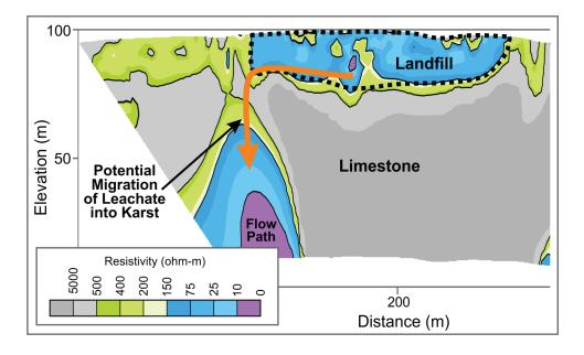
Aestus' GeoTrax Survey™ scanning technology was used to delineate the landfill boundaries as well as the geologic conditions beneath the landfill to a depth of about 100 meters. The graphic above shows:
