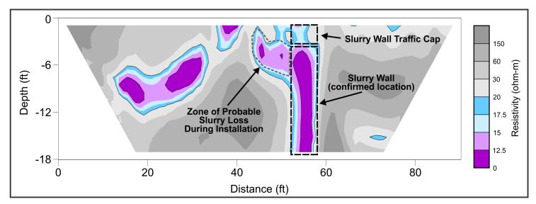
Slurry walls can be observed on a one time basis to evaluate if flow is moving beneath or laterally around the wall. Additionally, temporal observations can be used to test the installation effectiveness of the wall and it's effectiveness over time. This is especially helpful if the wall is a permeable reactive barrier and the flow dynamics need to be assessed.
