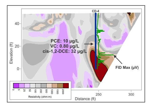
Aestus' subsurface imagery allowed for targeted confirmation drilling (CD-4; see above graphic) and collection of groundwater chemistry data as well as flame-ionization detector (FID) data. These multiple supporting lines of evidence indicated the resistive anomaly was primarily caused by the presence of methane gas:
