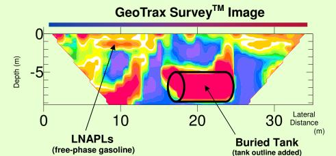
Aestus performed our GeoTrax Survey™ to determine potential environmental liabilities at this abandoned gas station site. We discovered a previously unknown buried tank (see image above). The client removed the leaking tank and impacted soils before construction began on this redevelopment project.
