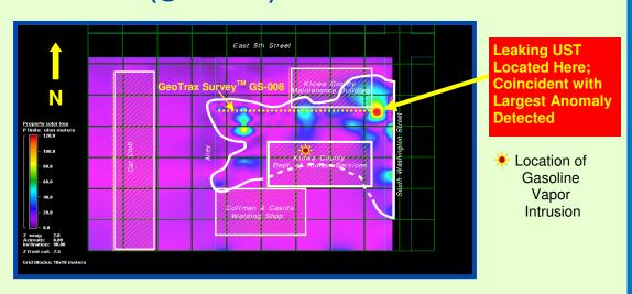
The plan view map above was generated using the Aestus' data showing the distribution of LNAPL at 15 feet below the ground surface. The source of the vapor intrusion (leaking UST) was located using our survey data.
