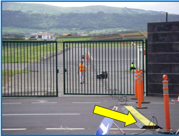
Photo of GeoTrax Survey™ transect crossing road at military base; geophysical cables under yellow/black traffic ramps (see yellow arrows)
